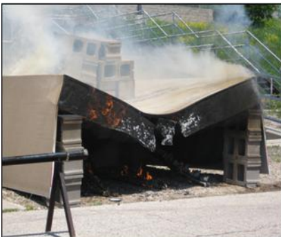
Untreated structure: Underside fully engulfed in flames within 5-minutes. Initial failure took place at about the 18-minute mark.
