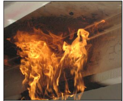
Treated structure: No flame spread from point of origin, demonstration ended at 38-minute mark with no evident structural fatigue.
