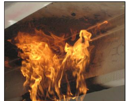
Treated structure: No flame spread from point of origin, demonstration ended at 38-minute mark with no evident structural fatigue.
